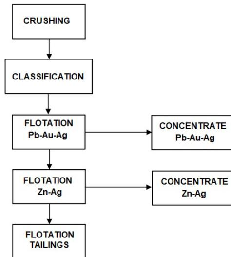
Figure 5.4 Schematic flow diagram, Mally Plant
