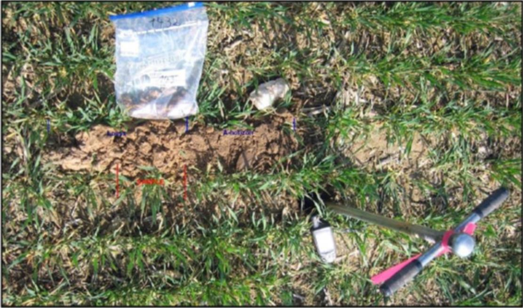
Figure 10-1 Soil sampling showing the sampled interval representing the subsoil (B horizon)
